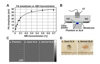
**Fig. 3** (A) Amplitude of photoacoustic signal versus concentration of methylene blue dye at a pseudolymph node. (B) Setup for *ex-vivo* estimation of concentration. (C) Photoacoustic B-scans of the phantom, the dyed SLN, and the normal SLN. The concentration in the phantom is ~0.07%, and the dyed SLN was estimated to be the same concentration. (D) Photographs of SLNs with (left) and without (right) dye deposit. ultrasonic transducer, UG: ultrasonic gel, and Wc: Water container.
