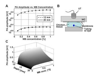
**Fig. 2** (a) Amplitude of photoacoustic signal versus concentration of methylene blue dye at 12- and 20-mm depth in chicken breast tissue, respectively. (b) Experimental setup for sensitivity measurement and *in vivo* estimation of concentration. (c) Estimation of concentration at 0- to 20-mm depth. UT, ultrasonic transducer; and WC, water container.
